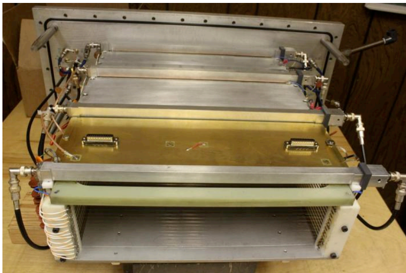
FIG. 2. Oxford detector with the new Anode mounted.
